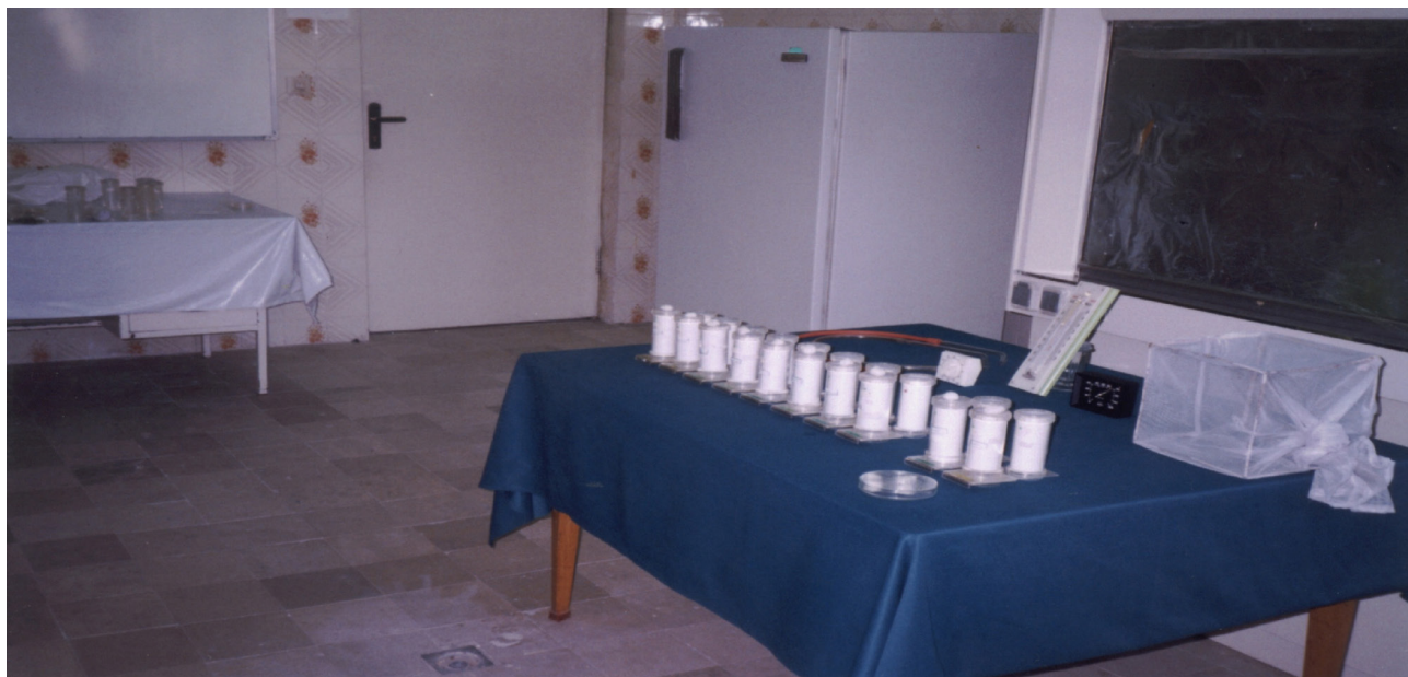
Figure 2: WHO protocol (Insecticide impregnated papers) for evaluation of insecticide resistance in mosquitoes
