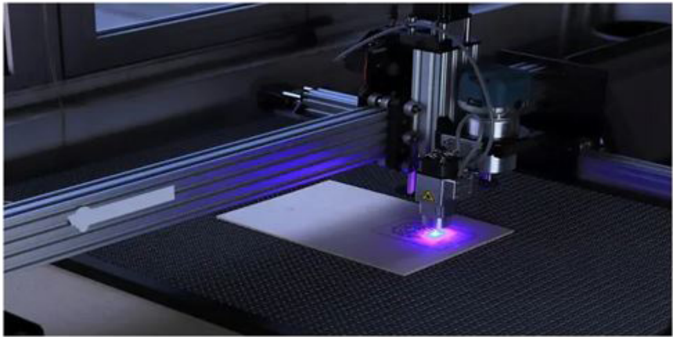
Figure 2 (b): shows the image of laser beam spot area with the mechanical device designed to modify the focused area of CO 2 onto the irradiated textile sample
