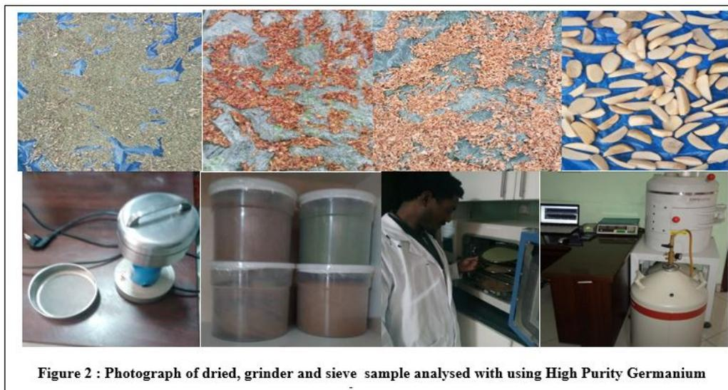
Figure 2: Photograph of dried, grinder and sieve sample analysed with using High Purity Germanium detector
